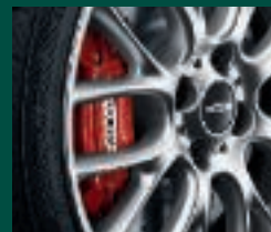
Sport brakes, 17 inches, with perforated and slotted brake discs
