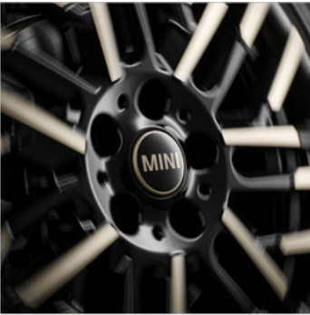
MINI floating hub cap. It is fixed. The innovative floating hub cap does not turn with the wheel. This way, the MINI logo also remains horizontal while driving.
