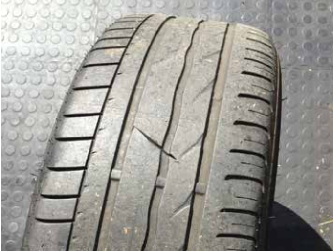
Example of a road legal / worthy tyre. Tread limit above 1 mm.
