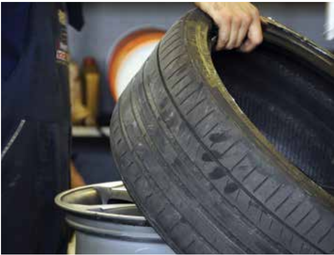
Example of a non-roadworthy tyre. Tread limit below 1 mm.
